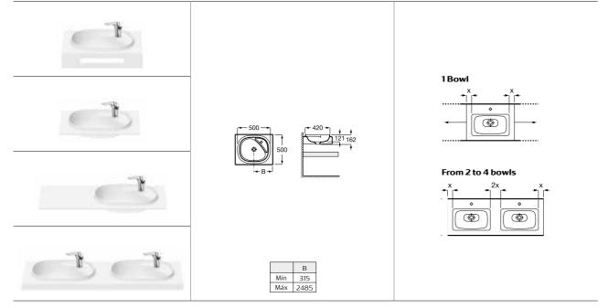
Wihtout overflow, fixed waste. Surfex  $\!\!^{\otimes}$  cover included. Dimensions in mm.
