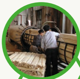
Untreated bamboo strips can be lightly steamed (Ecrú) or more intensely steamed (Caramel)
